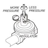
Fig. 3 Adjust gas pressure
